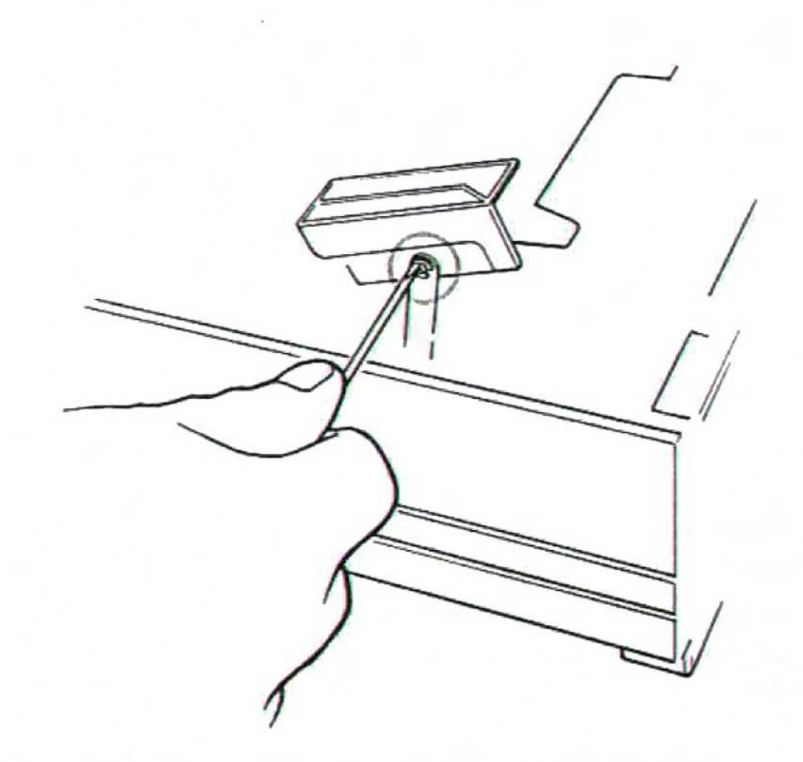
Fig. 3.5 Removing the circlip on the locking arm
