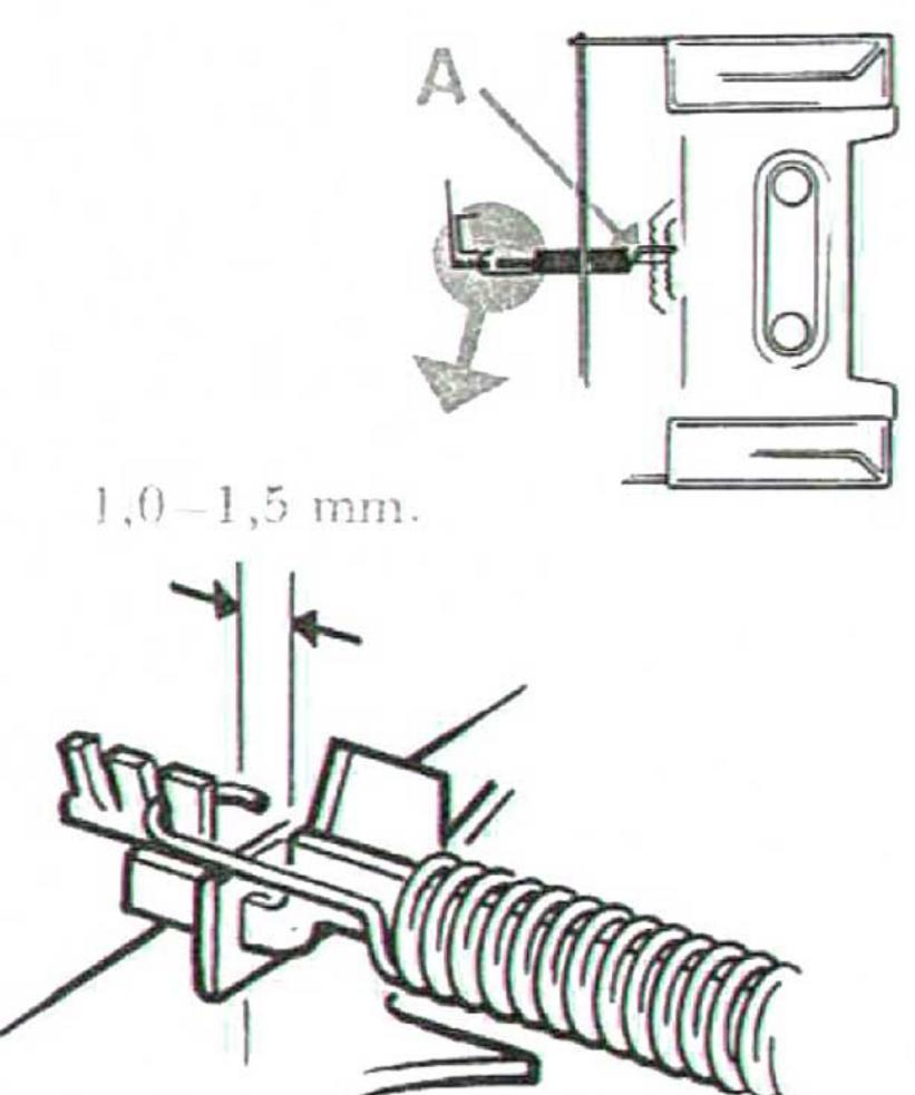
Fig. 3.12 Clearance on the tension spring
