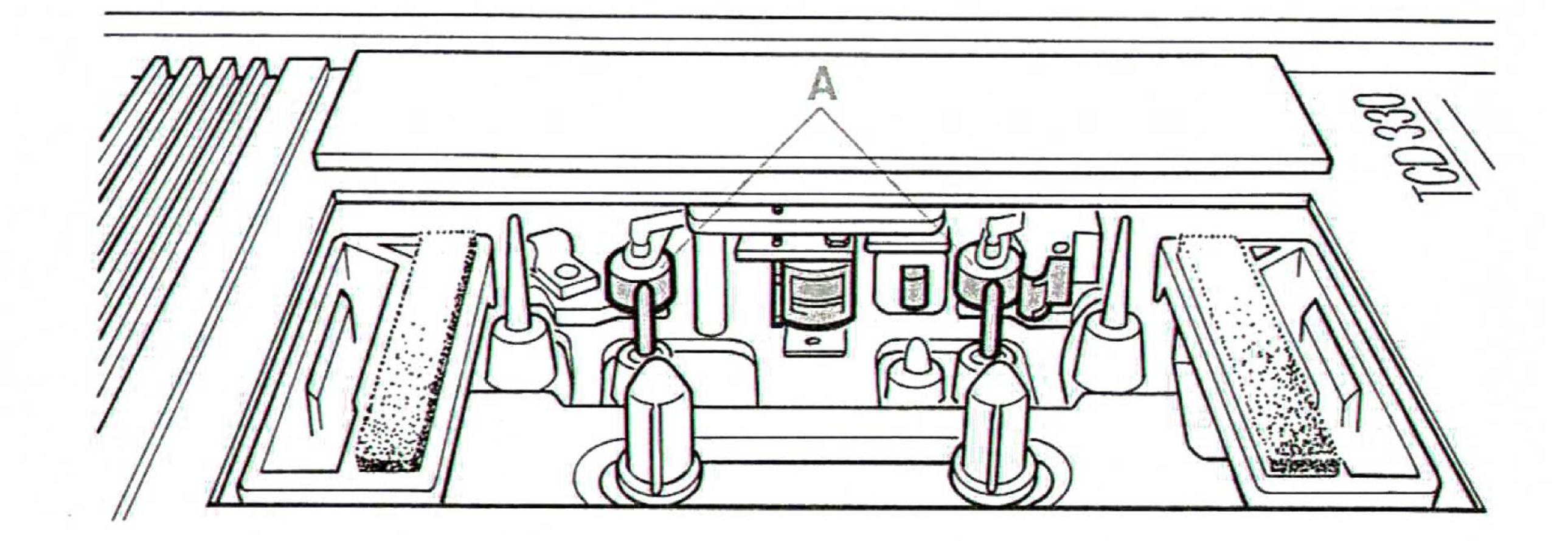
Fig. 2.1 Cleaning the tape path
