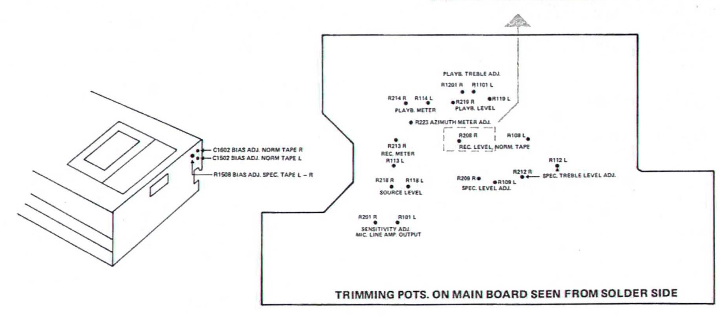
Fig. 6.1 Trimming pots. and Dolby encoders measurement points
