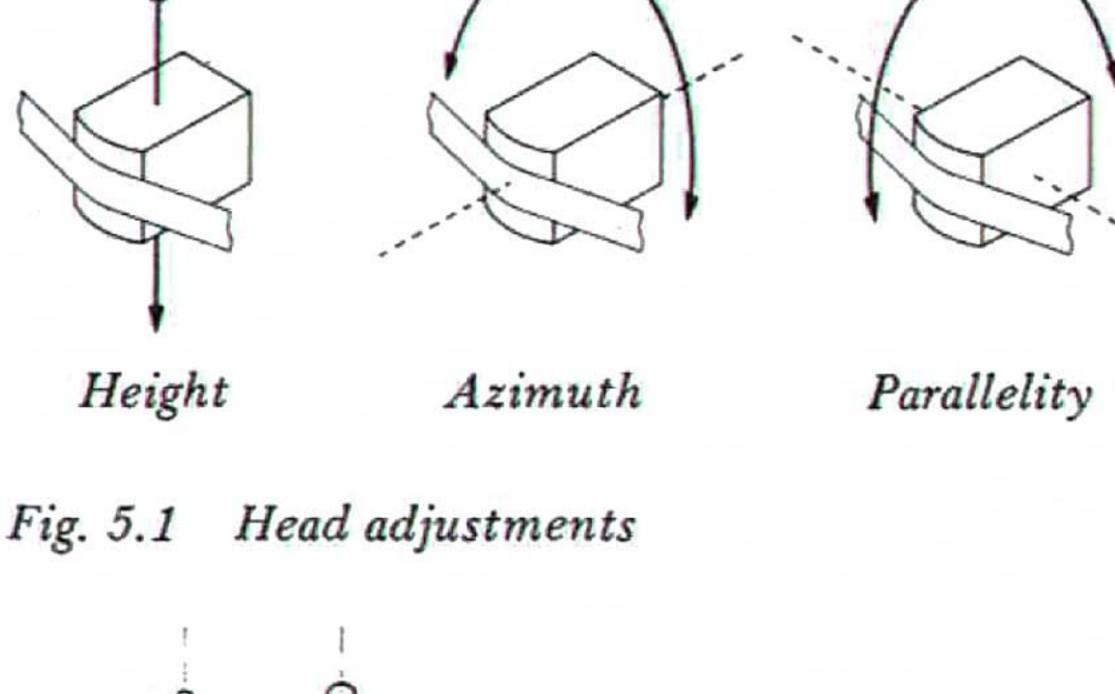
Lay a piece of white paper behind the pinch roller to make it easier to see the parallelism. Push the head bridge into the PLAY/RECORD position and check that the pinch rollers meet the capstans is a parallel fashion, see Figure 5.2. If necessary, adjust the HP screws shown in Figure 5.4.
