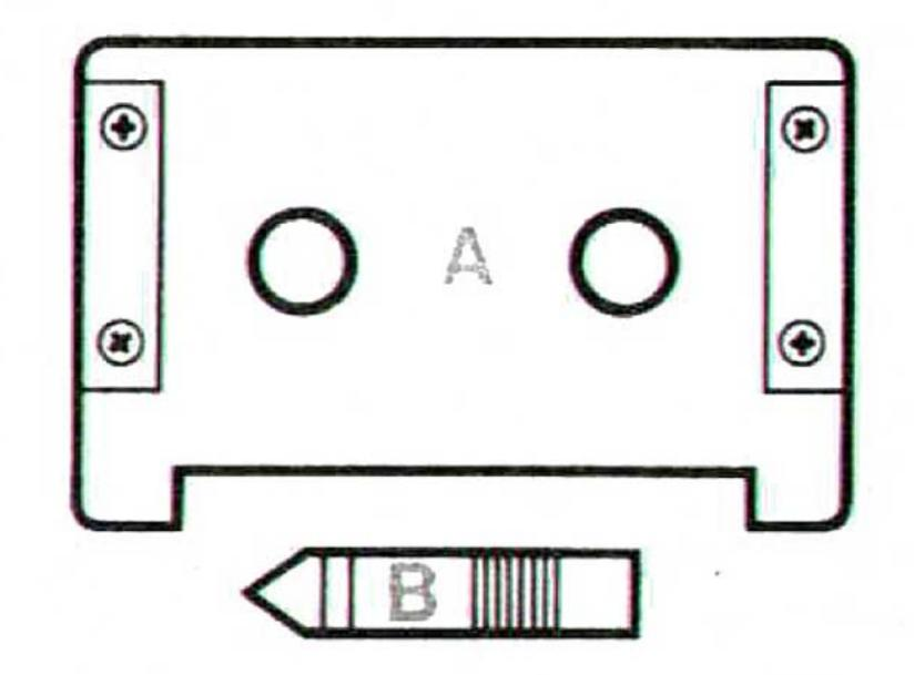
Insert a Tandberg test tape No. 23 or a standard azimuth cassette. Adjust the screw marked Playback, azimuth in Figure 5.6 to obtain max. output measured on a VVM connected to the OUT-PUT or RADIO socket.
