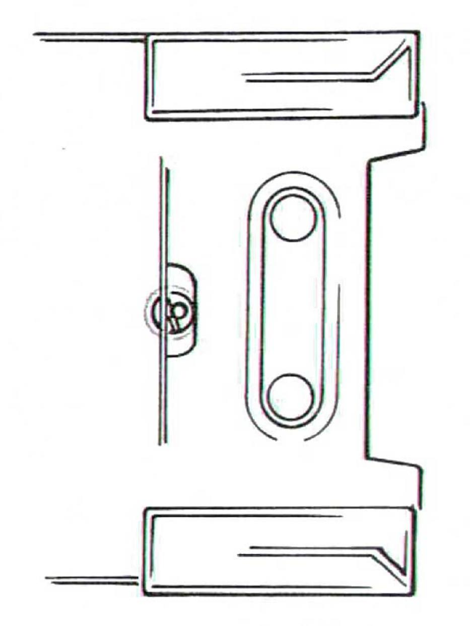
NOTE! Seal the eccentricity screw after the adjustment.
