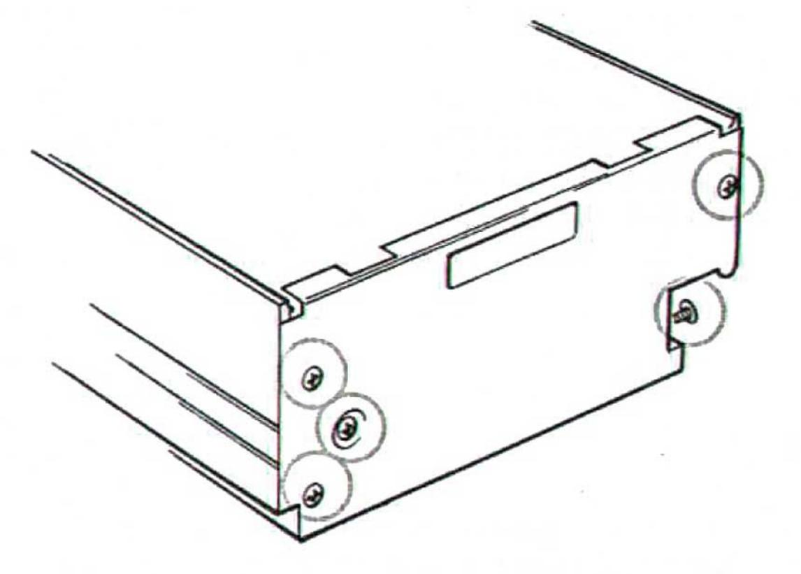
Fig. 3.6 Removing the right metal side panel
