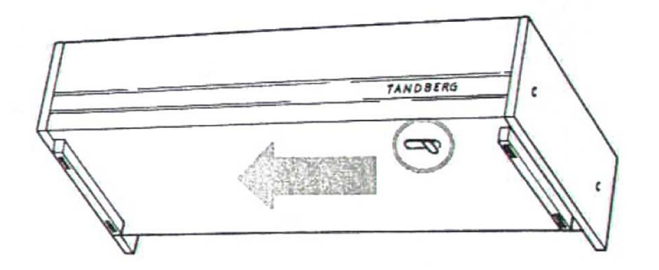
Pull the cassette compartment cover plate (with the coloured window) right off. Close the cassette compartment. Pull off the INPUT and OUTPUT knobs.
