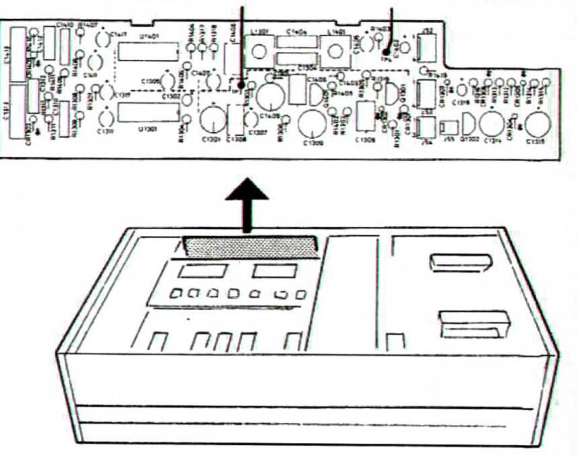
Apply 1000 Hz from the sig. gen. to one of the inputs. Reduce the level at the sig. gen. by 35 dB or reduce the level by a similar amount on the INPUT LEVEL controls.
