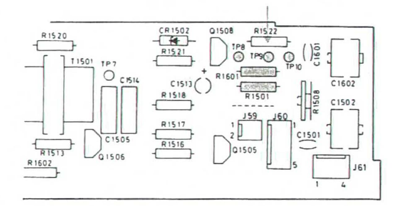
Set the machine to STOP and press down the REC. PRESET button. Set the DOLBY N.R. knob to OFF. Connect an audio sig. gen. to the INPUT or RADIO socket.
