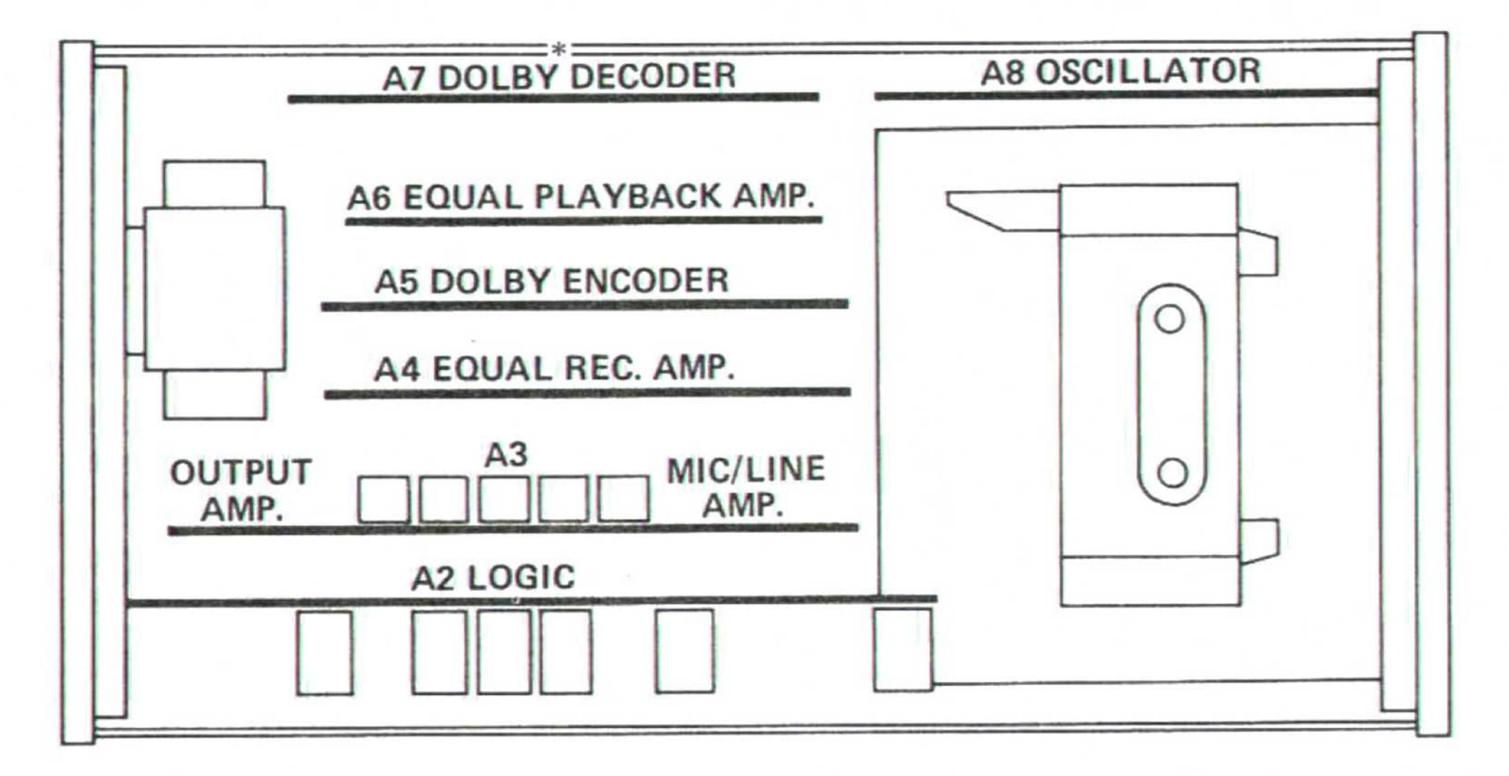
Fig. 4.1 Location of printed boards (meter board removed)
