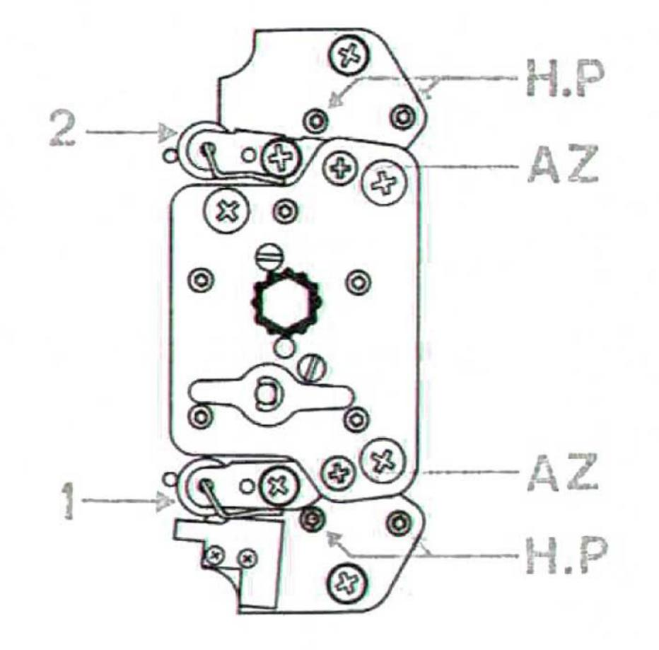
Fig. 5.4 Adjustments for the pinch rollers
