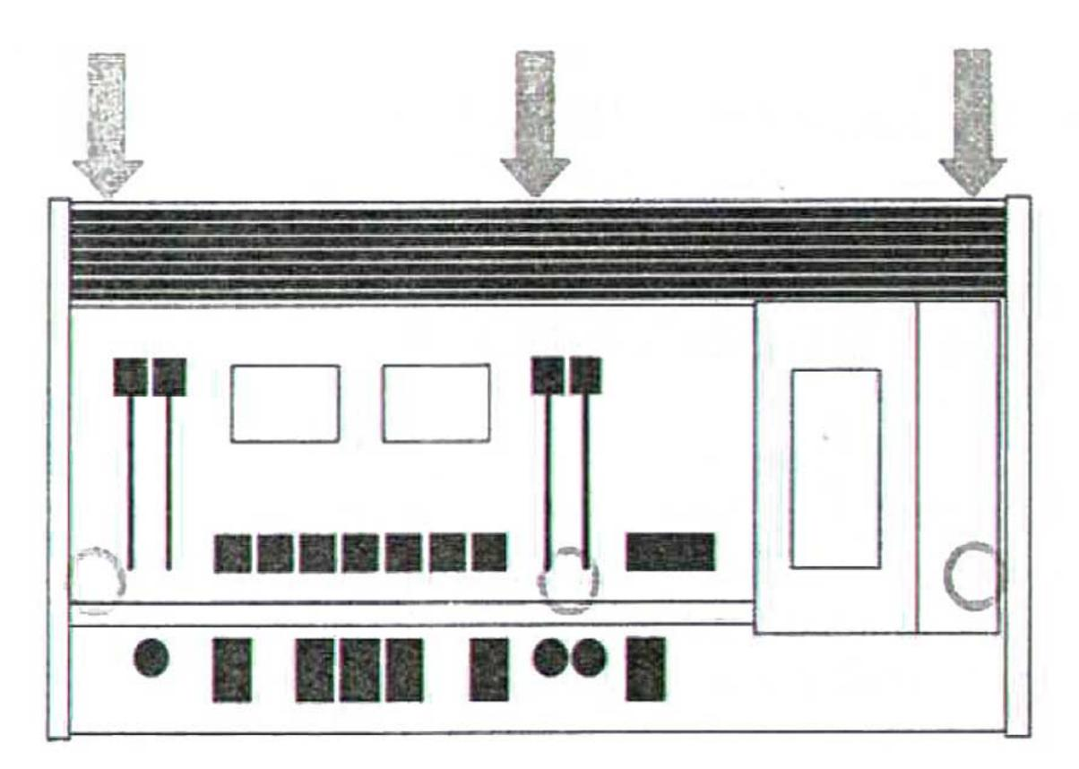
Fig. 1.2 Removing the top panel
